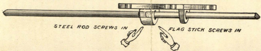
Showing back of Marker, and how Steel Rod and Flag Stick screws in.
